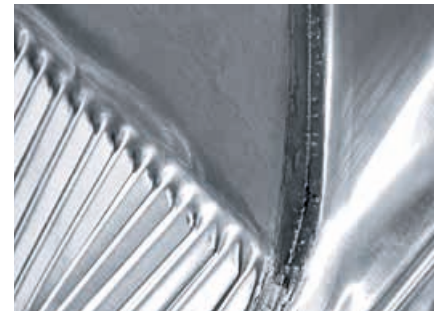
Completed soldered seam
