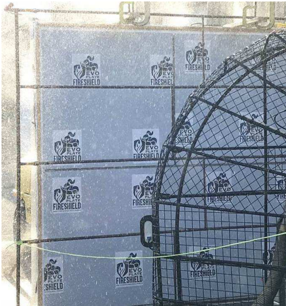
Figure 3 – AAMA 501.1, Dynamic Water Penetration Test
